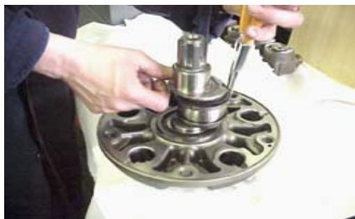
Dislodge the C-clip from the front-side of the spherical support ring[11].
