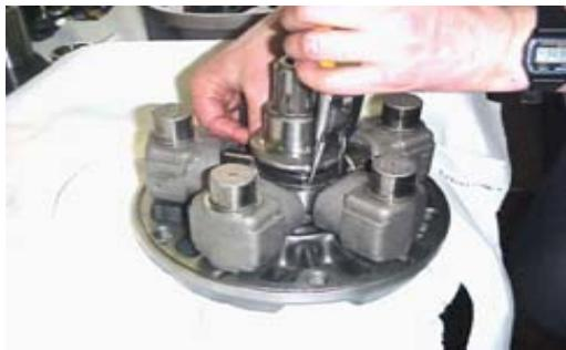
Turn the motor over so that the shaft points downwards, insert and tighten the motor casing closing bolts. Using an appropriate lever inserted in the distributor drive-pin slot ensure that the shaft rotates through 360 degree without resistance.
